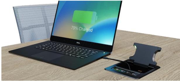
Connect the PSU to the VXT and provide your connected USB-C device with charging power up to 100W.
